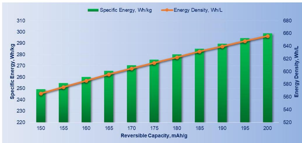
Figure 3. Specific energy and energy density evolution of cells with cathode materials of different capacities.
