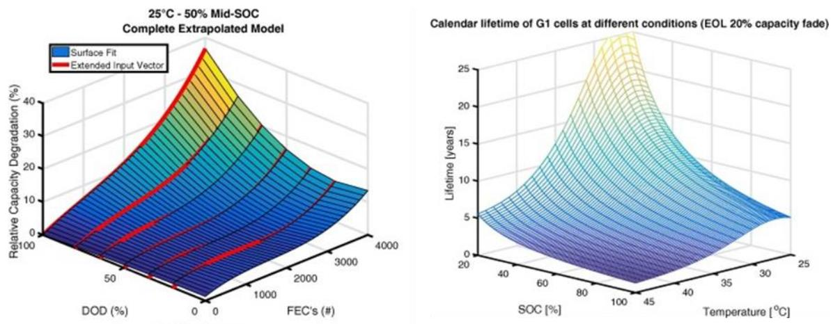
Figure 6. Simulated Cycle life (Left) and Calendar life(Right) of a high energy cell with NMC333 cathode[3].
