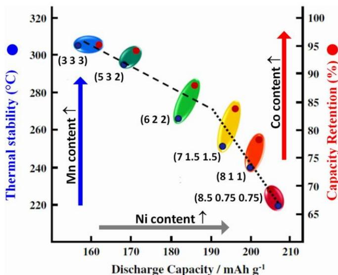
Figure 4. A map of relationship discharge capacity (black), thermal stability (blue) and capacity retention (red) of Li/Li[Ni<sub>x</sub>Co<sub>y</sub>Mn<sub>z</sub>]O<sub>2</sub> compounds with number in brackets corresponding to the composition (Ni Mn Co). [2]
