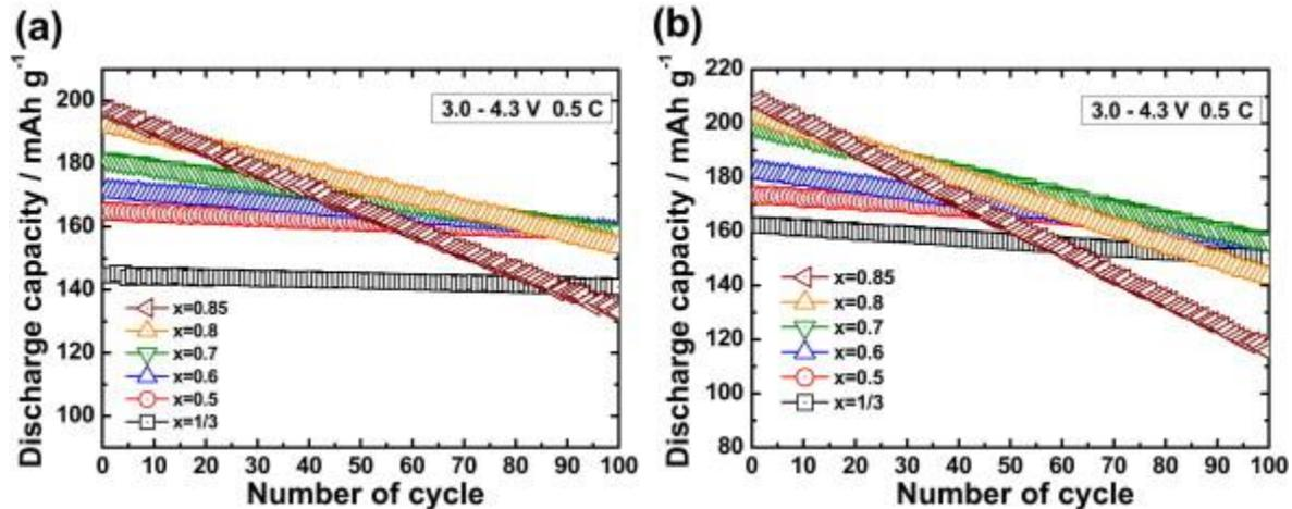
Figure 5. Discharge capacity vs. cycle number for the  $\text{Li/Li}[\text{Ni}_x\text{Co}_y\text{Mn}_z]\text{O}_2$  ( $x = 1/3, 0.5, 0.6, 0.7, 0.8$  and  $0.85$ ) cells at (a)  $25^\circ\text{C}$  and (b)  $55^\circ\text{C}$ . The Co and Mn contents are  $-y=1/3, 1/3, 0.2, 0.15, 0.1, 0.075$  and  $z=1/3, 0.2, 0.2, 0.15, 0.1, 0.075$ . [3]
