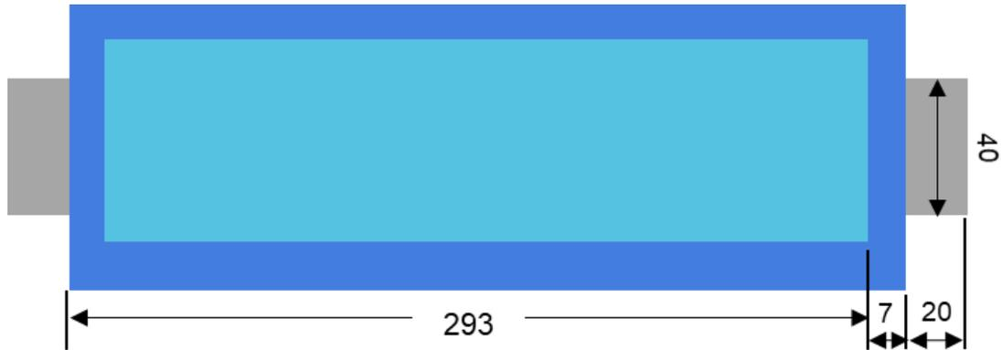
Figure 2. Schematic of the 60Ah high energy pouch cell used in Umicore model. All the dimensions are in mm.
