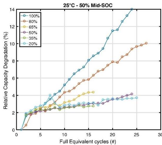
Figure 7. Cycle life evolution of a 20Ah cell with NMC333 cathode [3].
